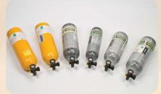
MSA offers a choice of three lowpressure (2216 psig) 30-minute-rated cylinders for use with this SCBA. Choose carbon-wrapped, fiberglass hoop-wound, or all-aluminum construction cylinders. High-pressure (4500 psig) carbonwrapped cylinders are available in 30-, 45- or 60-minute durations.
